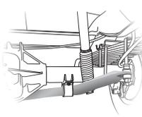
**HEAVY-DUTY FRONT & REAR STABILIZER BAR** A larger bar and polyurethane bushings, instead of rubber, transfer power faster for extra support, more stability and easier handling
